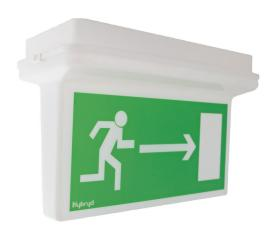
Emergency light fitting, wall or ceiling lights with a higher degree of protection IP53. The casing is made of plastic, white RAL 9003. Diffuser milky or transparent plastic. The light source is LED or fluorescent light.
