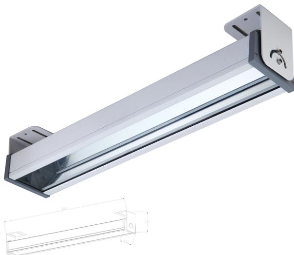
Small size IP65 LED luminaire, designed for surface mounting. Adjustable tilt up to  $\pm 45^\circ$ . Designed for halls, warehouses or open areas. The fitting is made of aluminum. LED light source obscured by tempered glass.
